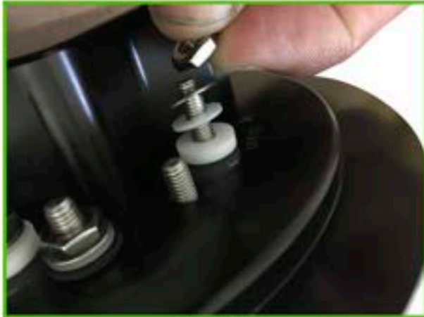
Step 27 Install one delrin washer, one stainless steel nut on the positive terminal isolator
