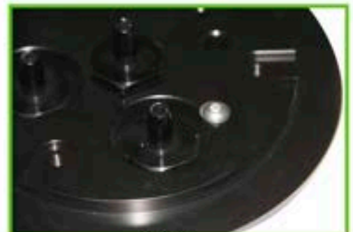
Step 8 Tighten till O-ring seats.
