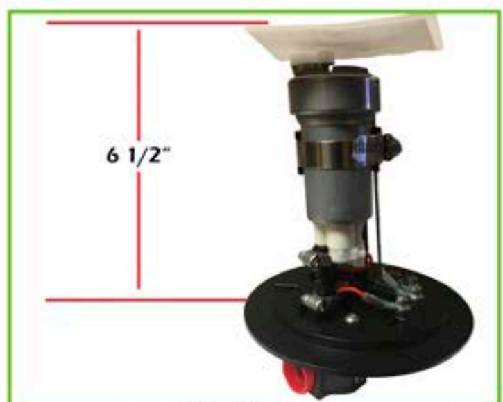
Step 32 Measure the base of the pump hat to the bottom of the filter. That will measure 6 1/2
