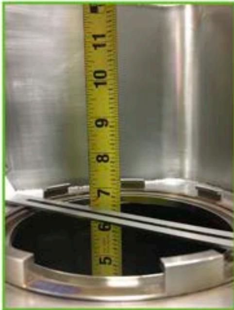
Step 1 Measuring the depth of the tank using a straight edge.
