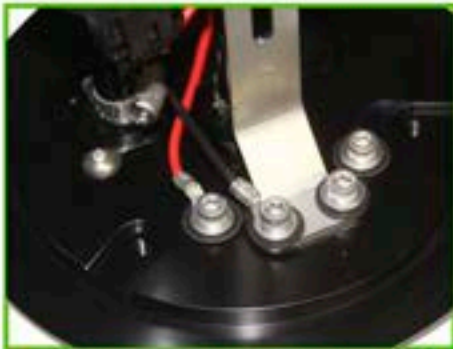
Step 29 Tighten all 4 till viton washer seats.
