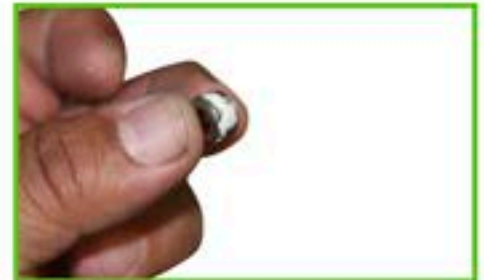
Step 2 Dab some Loctite 567 Thread Sealer or preferred sealer that you use.
