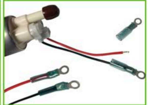
Step 24 Cut the harness to the desired length and install terminals. Apply heat to the heat shrink terminals.
