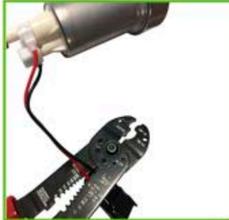
Step 24 Cut the harness to the desired length and install terminals. Apply heat to the heat shrink terminals.
