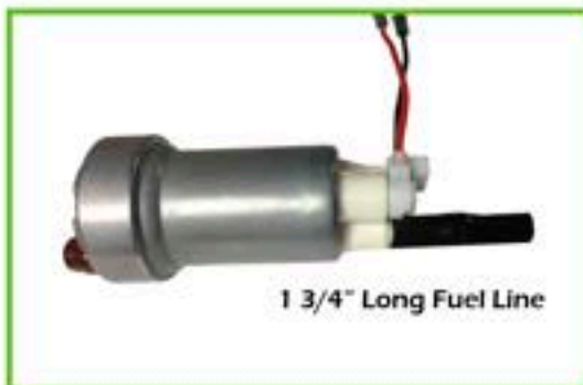
Step 21 Install the 1 3/4" Fuel Line on to the fuel pump
