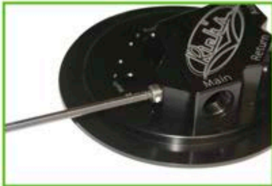
Step 3 Tighten the Steel Plug till flush with pump hat.
