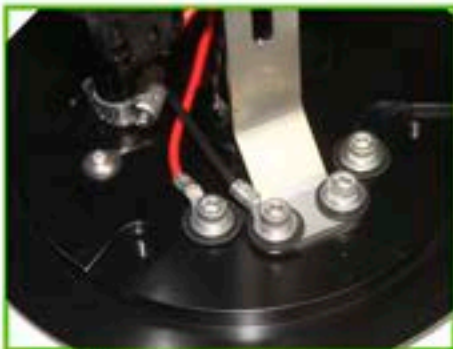
Step 29 Tighten all 4 till viton washer seats.
