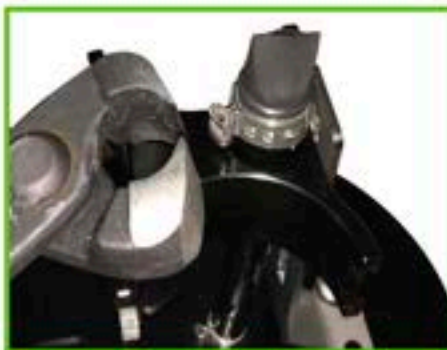
Step 20 Use Jaw Pincers to correctly pinch the clamp.
