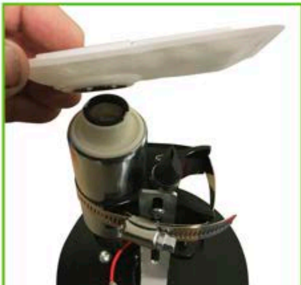
Step 31 Install fuel pump filter
