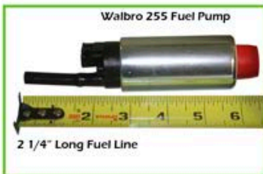
Step 21 Install the 2 1/4" Fuel Line on to the fuel pump
