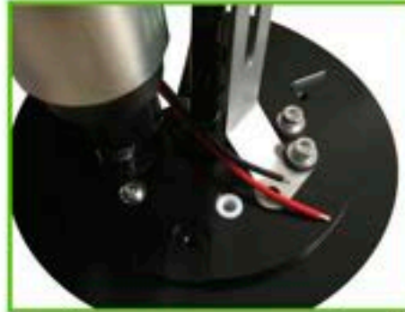
Step 24 Cut the harness to the desired length and install terminals
