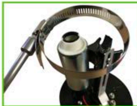
Step 30 Install clamp over the pump hanger and bracket then tighten
