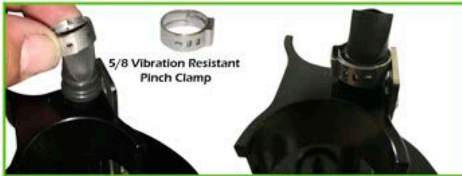
Step 19 Install the 5/8 Vibration Resistant Pinch Clamp
