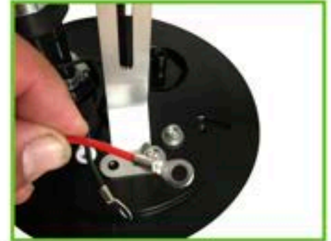
Step 24 Cut the harness to the desired length and install terminals
