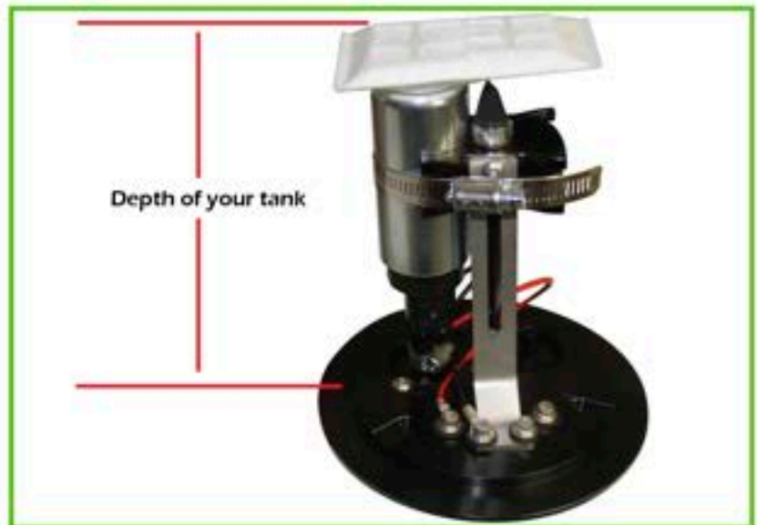
Step 32 Measure the base of the pump hat to the bottom of the filter. That should be the same as the depth of your tank. Now it's ready to install into the tank.
